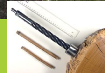
A researcher uses a borer to extract a core from a living tree. Inset: Various drills used for boring.
