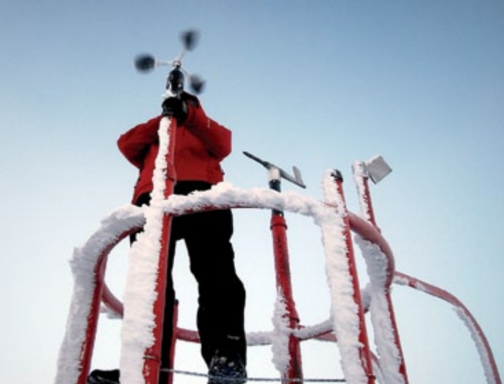
Clark adjusts the three-cup anemometer, which is used to measure low wind speeds.
