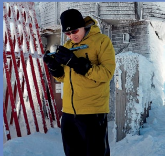
Clark braves the elements to read the sling psychrometer, which measures the amount of water vapor, or humidity, in the air.
